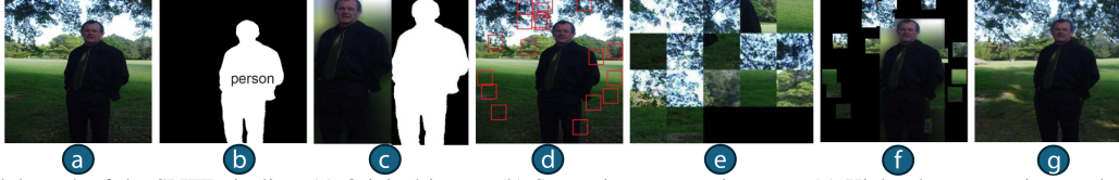
Fig. 8. Visual walkthrough of the SPIFF pipeline. (a) Original image, (b) Semantic segmentation map, (c) High-relevance region mask, (d) Patches sampled from background, (e) Patch grid from sampled patches, (f) Combined data for reconstruction, (g) Final reconstructed image.
